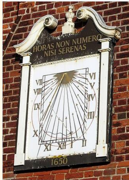
SSW facing, vertical declining sundial on the Moot Hall in Aldeburgh, Suffolk, England. The gnomon is a rod that is very narrow, so it functions as the style. The Latin motto loosely translates as "I only count the sunny hours."
