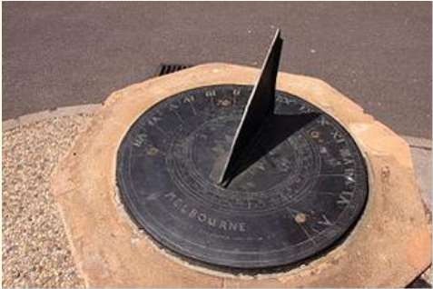
A horizontal dial commissioned in 1862, the gnomon is the triangular blade. The style is its inclined edge. [1]
